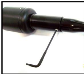
7. Screw in two (2) 512-M4X6SS316P grub screws to secure the cable and the sensor with supplied Allen key
