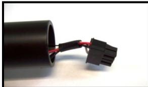
1. The sensor connector is exposed and ready to connect to the cable connector.
