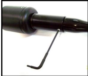
2. Remove the two (2) grub screws (Greenspan part #512-M4X6SS316P) using the Allen key supplied. (N.B Allen key is supplied in spare parts kit with original packaging)
