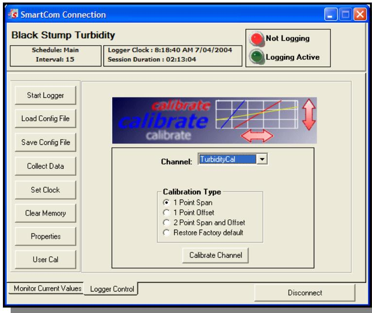
Allows re calibration of channels within the logger.
