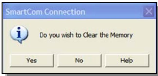
This control is used to clear the contents of the Data Logger Memory.
