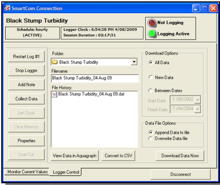
This allows collection of the logged data. Various options allow collection of all Data, New Data or Data between specific dates. Data can be downloaded to new files, or appended to existing files.
