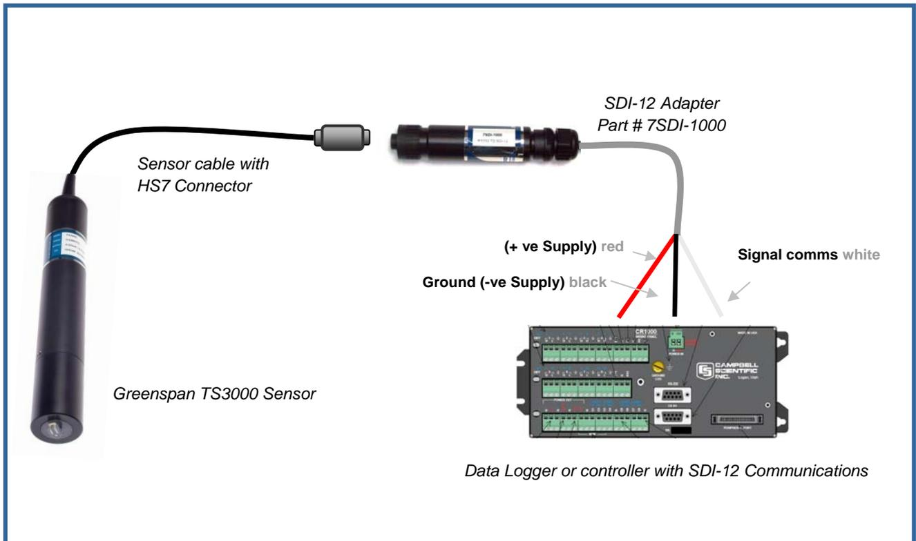
**Typically the sensor will be connected to a Data Logger or Process Controller which will provide the power and ground connections and provide connections for serial SDI12 output.**
