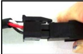
3. Once connectors are completely pushed together, the rocker arm on the sensor connector will clip in with the cable connector and secure the connection.
