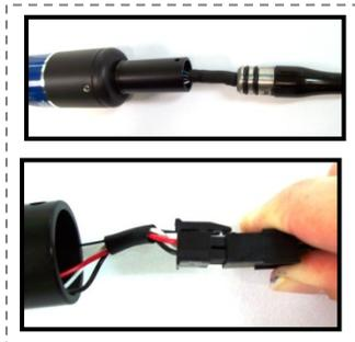
3. CAREFULLY pull tube away from cable mould. Once the tube has been pulled away from cable mould, the connector will be revealed as pictured left.
