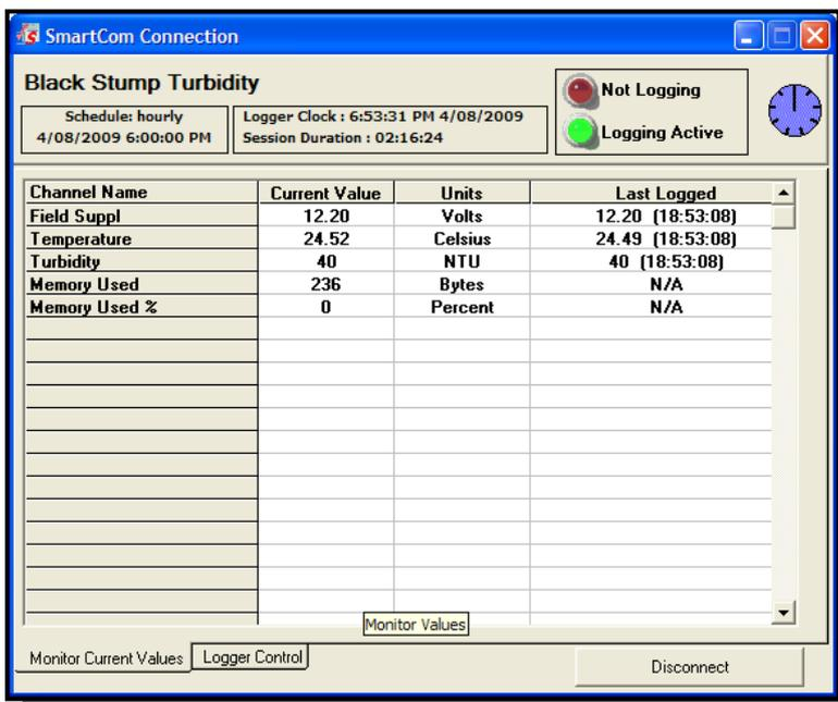
Confirm Logger is operational by checking the following:
