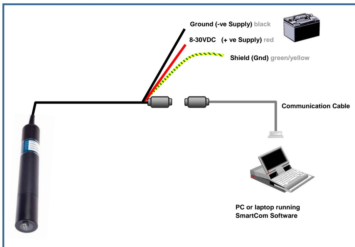
The SmartCom software provides for configuration of the data logger, collection of logged data, and all other functions. The Greenspan Aquagraph software provides graphical and tabular presentation of logged data and export to spreadsheet format. A brief description of the key components of the SmartCom software is included in this manual. A fully documented online help function is also included within the SmartCom software. It can be started by Hitting F1 key.
