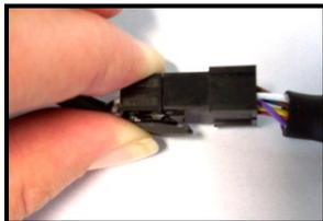
4. Release locking device on the connector by gently pinching rocker arm on the cable connector and pull apart.
