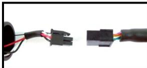
2. Align the cable connector with the sensor connector and push together. The connector is polarized and will only fit together one way.
