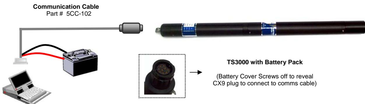
*TS3000 is a complete logging turbidity sensor. Communication and configuration of the sensor is via the SmartCom Software on the supplied CD.*
