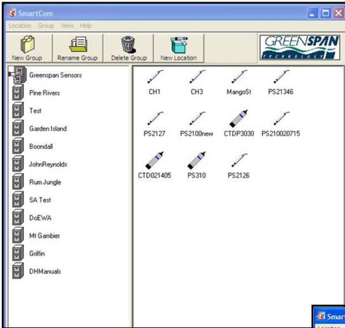
The Main Screen is divided into 2 Panels. The left side shows the Groups. The right side shows the locations within each Group. (The concept allows all sensor sites to be put together into logical groups – eg by catchment, area, client, sensor type etc)
