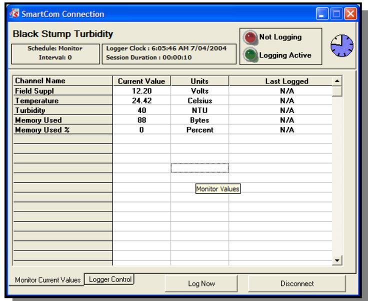
The Logger Control Screen provides access to all configuration, Data retrieval, Logger management and Calibration routines.
