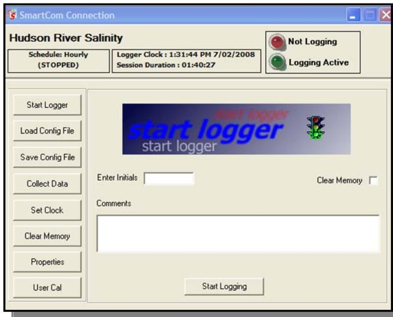
When starting the logger –the user is able to enter comments, and is given an option to clear memory.
