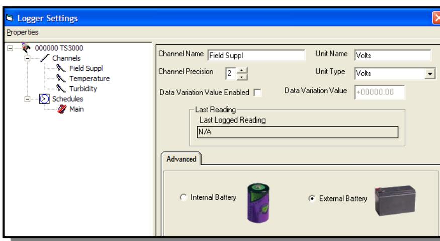
The Sensor will be powered by some type of DC (12-24V) power supply which may be either an internal battery pack or an external battery system. The user must click and select the correct battery type to ensure accurate battery life & voltage calculations.
